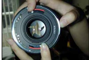
exposes the entire frame at once compared to focal plane shutters that exposes the frame in a top/down or right/left sequence that exposes in a partial fashion over the course of the shutter speed being used. There is a mechanical limit that manufacturers have not been able to push beyond 1/300 in the Nikon F5 and Minolta Maxxum 9 cameras.
